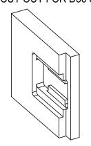
IMPORTANT: Please reference the cut out depth from the top panel surface. Ensure that the cut out depth is exact and does not change with panel thickness variations
