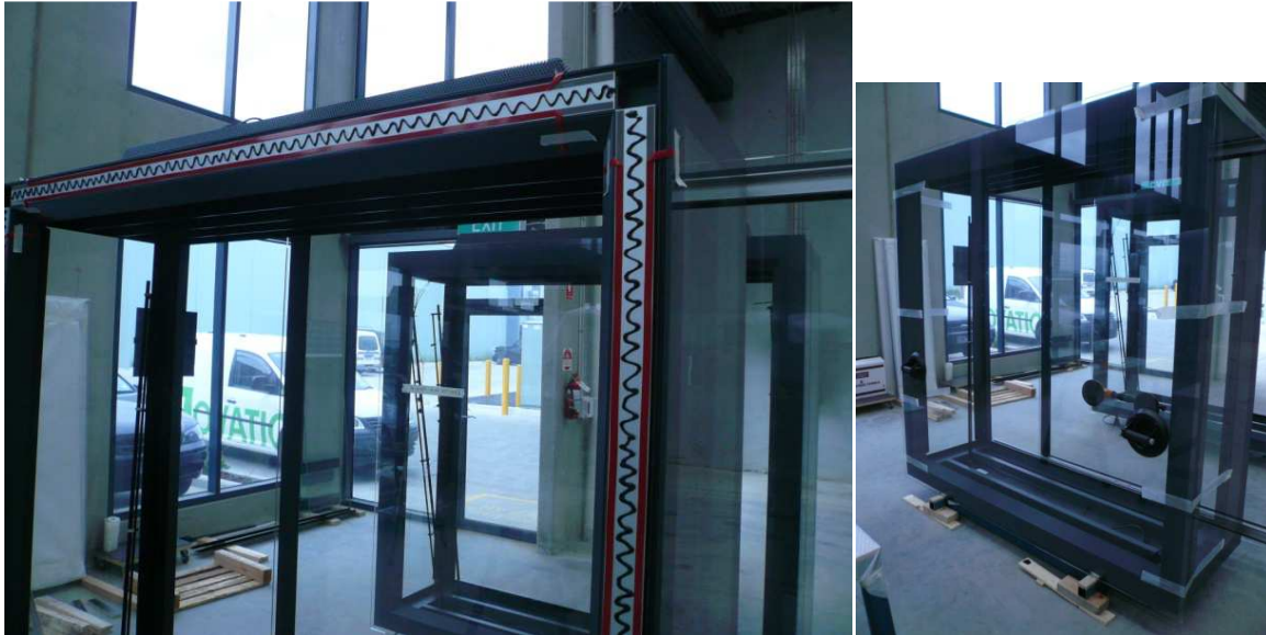
High-Tech-Tape is visible with the red lines.
